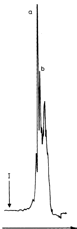
Figure. Crude porphyrin a dimethyl ester derived from haem a dipyrrolic complex (see text) fractionated by h.p.l.c. on two 10 \mu C 18 Bondapak columns in series with degassed acetonitrile as solvent. Flow rate 2.5 ml min -1 at ca. 2 500 lb in -2 with a u.v.-visible analyser set at 412 nm. I = Injection point, peak a is porphyrin a dimethyl ester, peak b is the porphyrin of molecular weight 862 (see text)
